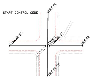
**Note:** It is not mandatory that string identifiers be used. This is only necessary if you wish to collect data using identical feature codes and need to develop multiple strings simultaneously. Examples of this may be when surveying in a crisscross fashion and wish to collect multiple 1310 (edge of oil) strings. If surveying in a linear fashion (collecting the entire length of the physical feature) a code such as 1310 st could be used and reused when moving from one pavement edge to another
