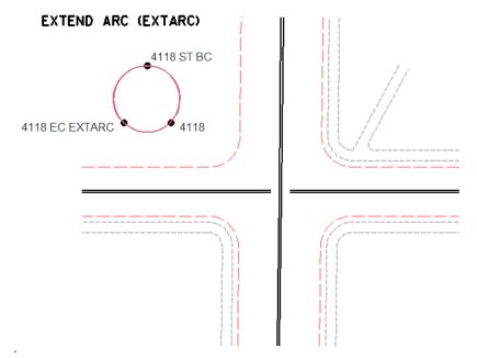
**Note:** When the feature is pushed to a DTM the feature will not keep the circular shape. The DTM feature will be made up of two line segments.
